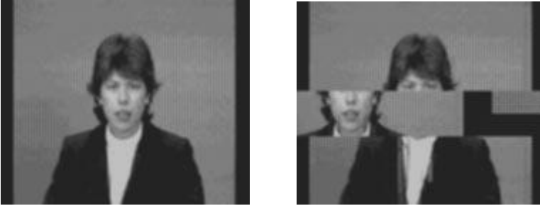
Fig. 3.3. Sent vs received video frame with 3 directly lost macroblocks during transmission
